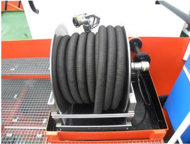
Fuel supply winch
